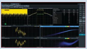
▲ Fig. 1 Amplifier characterization featuring both frequency and time domain data.
