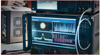
▲ Fig. 1 Example of scopes, signal analyzers and signal generators.
