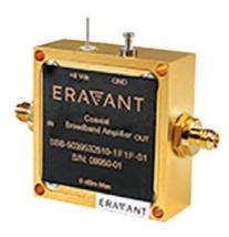
SBB-5039532510-1F1F-S1 is a 1 mm broadband amplifier with a typical small-signal gain of 25 dB, a nominal P1dB of +10 dBm and a typical noise figure of 7.0 dB across the frequency range of 50 to 95 GHz. The DC power requirement for the broadband amplifier is +8 VDC/300 mA. The use of a heat sink is advised to assist in cooling the device. The RF connectors are female 1 mm connectors. Other port configurations are available under different model numbers.
